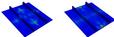
Figure 1: Guided ultrasonic waves in carbon fibre composite.
