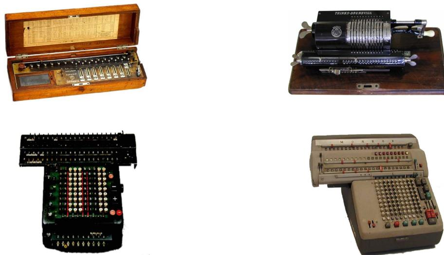
**Fig. 5.** Mechanical computing devices equipped with the desired capability: **Burkhardt Arithmometer**, Glashütte, Germany, 1878; **Brunsviga**, Braunschweig, Germany, 1917; **MADAS**, Zürich, Switzerland, 1936; **MONROE**, New Jersey, USA, 1956.
