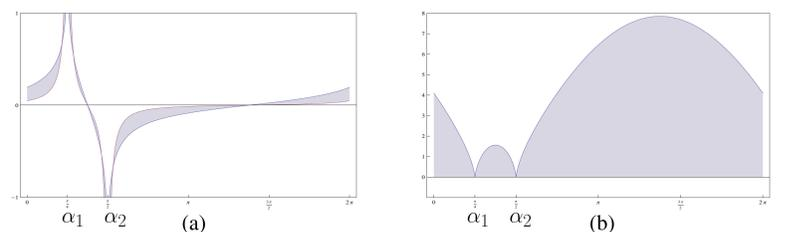
Figure 3: (a) Analytical trace  $u_3|_{\partial\Omega_2}$  for a cylinder (red) and  $u_2|_{\partial\Omega_2}$  for a disc (blue); (b) Corresponding multiplier function  $h$  defined in (3); Applied current pattern: source at  $\alpha_1 = \pi/4$  and sink at  $\alpha_2 = \pi/2$
