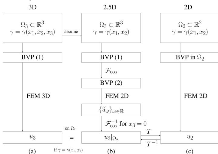
Figure 2: Comparison of 3D, 2.5D and 2D forward problem. The data transformation  $T$  represents a bridge between the 3D procedure in (b) and the 2D procedure in (c).
