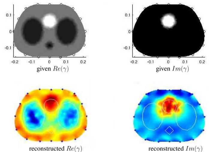
Figure 4: Reconstruction result for thorax model including heart, lungs and backbone. 16 electrodes and noise free measurement data as dipole-dipole configuration are applied. Reconstruction algorithms: Tikhonov-regularised Gauss-Newton method
